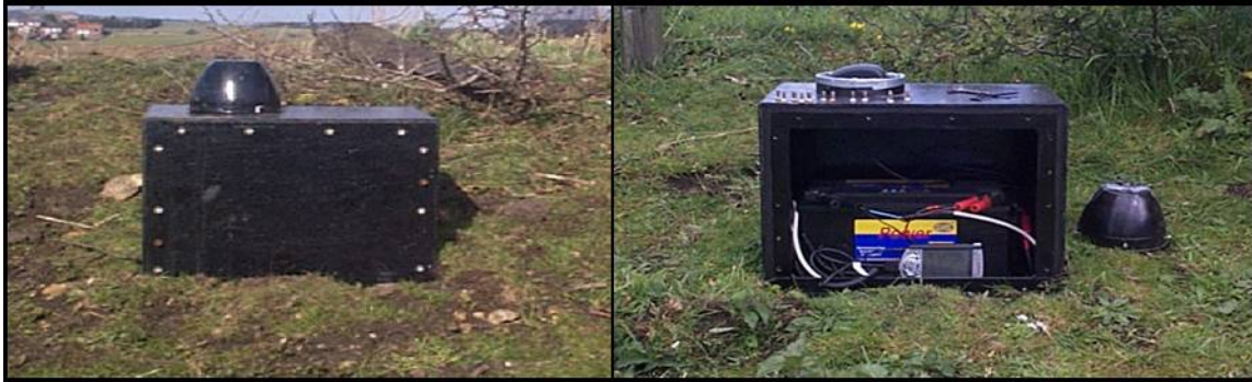
Figure 3. GPS remote monitoring system prototype.
