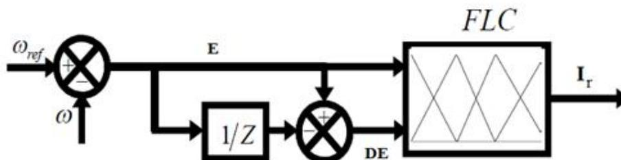
Fig. 3 Schematic model of fuzzy logic controller
