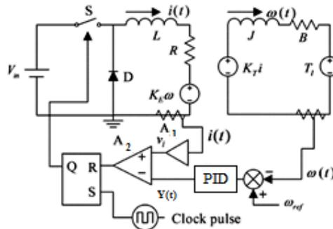
Fig. 2 Equivalent circuit Current-controlled DC drive system
