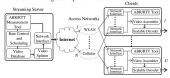
Fig.1. Sample system architecture of a scalable video streaming system with clients and access networks.
