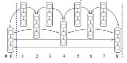
Fig. 2. Dependency among NALUs of H.264/SVC streams. Each square rep- resents an NALU belonging to an MGS layer, and each rounded rectangle rep- resents a video frame.
