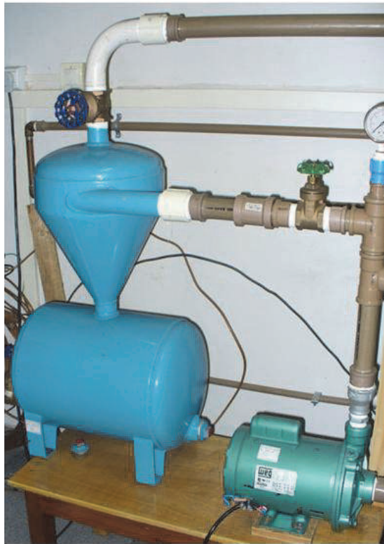
Fig. 8. Hydrocyclone system (with hydraulic pump) used to separate the charcoal from the SCBA. The charcoal with water goes out of the hydrocyclone through the vortex finder (overflow) and the inorganic components go to the tank (reservoir) through the spigot (underflow)
