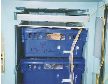
Figure 4 - Validation of an Insulated Eutectic Container
