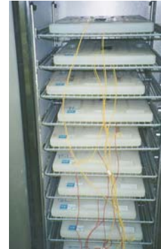
Figure 5 - Freezing Down Eutectic Plates
