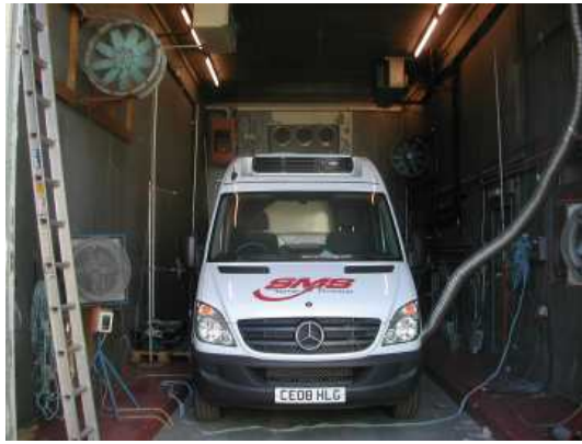
Figure 8 - Refrigerated Vehicles Undergoing Summer PQ Testing in the CRT Test Chamber
