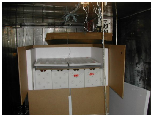
Figure 3 - Thermal Validation of a Pallet Shipper
