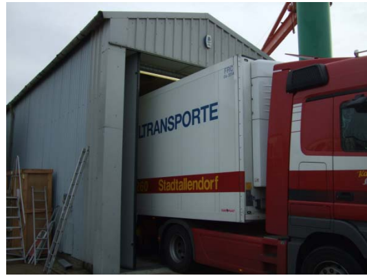
Figure 8 - Refrigerated Vehicles Undergoing Summer PQ Testing in the CRT Test Chamber
