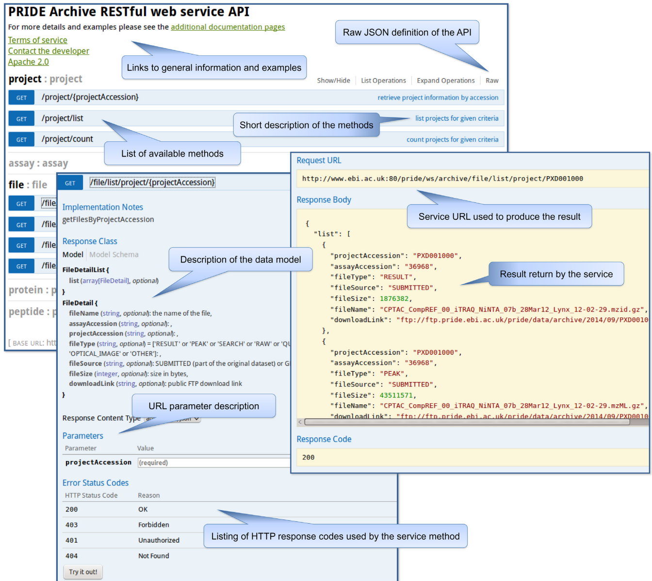
Figure 2. Schema of the interactive documentation of the PRIDE Archive web services implemented using the Swagger™ framework.
