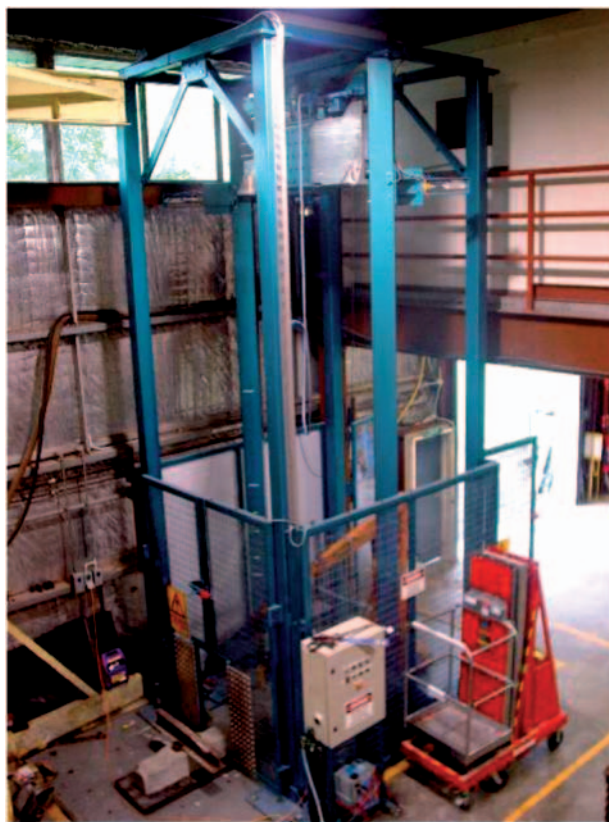
Fig. 4 New high-capacity drop-weight impact testing machine at the UoW
