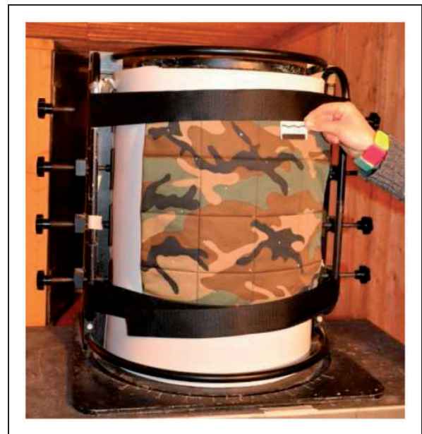
Figure 3. Typical specimen mounted for ballistic testing.
