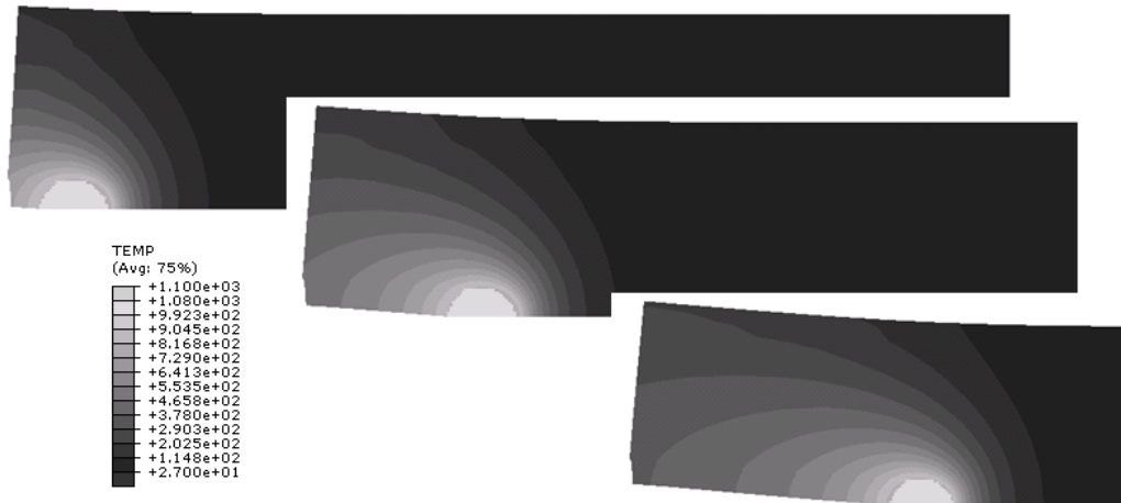
Fig. 12: temperature field over the distorted mesh (displacement magnified by a factor 5) when the nodes are relaxed behind the weld pool simulating the propagation of a hot tear.
