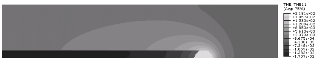
Fig. 9: Thermal strain distribution when the electron beam is located at x = 60 mm.
