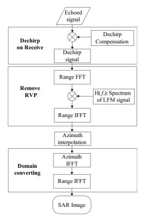
Figure 4. Flowchart of the conical-trajectory PFA.
