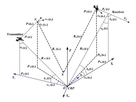
Figure 1. Spotlight bistatic SAR geometry.
