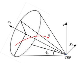
Figure 3. Schematic figure for conical trajectory.
