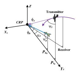
Figure 8. The bistatic forward-looking geometry used for simulation.
