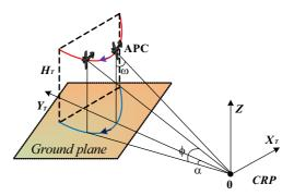
Figure 5. Hyperbola trajectory for the fixed altitude mode.
