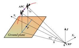
Figure 6. Ellipse trajectory for the linear ground-projection mode.
