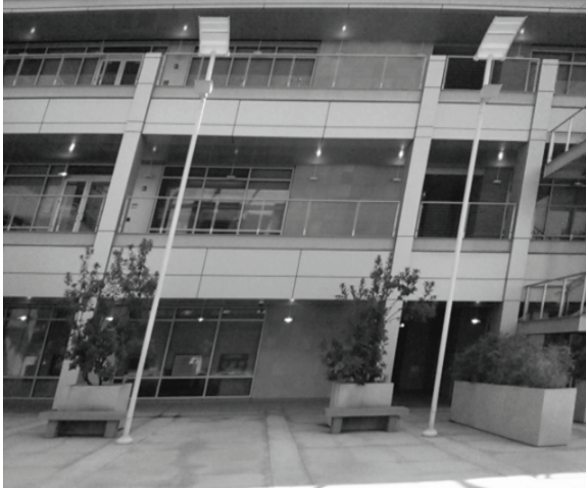
Fig. 1. An example image with rolling-shutter distortion.
