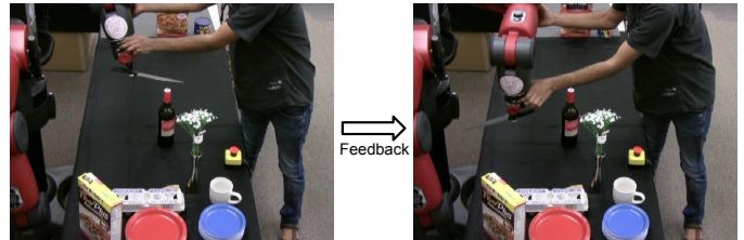
Fig. 8: Feedback to RoboBrain. RoboBrain also improves with feedback provided on physical robots. In this figure user provides feedback on robot by improving the trajectory proposed by the RoboBrain. As feedback user moves the knife away from himself.
