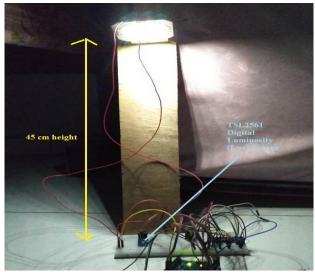
Fig. 7.PWM-LUX experiment setup
