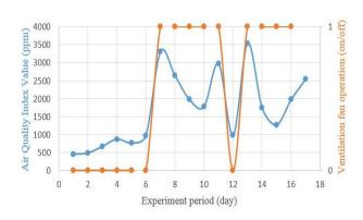
Fig. 10. Recorded AQI and Ventilation System Operation
