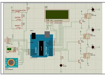
Fig. 5.Project simulation circuit
