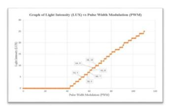
Fig. 8. Relationship between PWM and LUX
