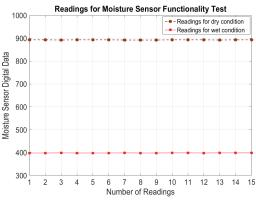
Fig. 10. The result for the functionality moisture sensor test
