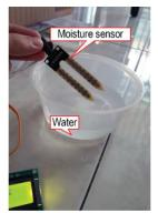
Fig. 8. Moisture sensor test for dry condition
