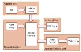
Fig. 1. Functional block diagram
