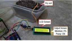
Fig. 11. LCD Output based on dry soil condition
