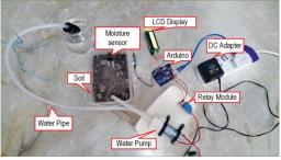
Fig. 4. Hardware implementation for the automatic irrigation system (Top view)
