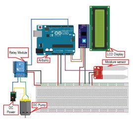
Fig. 3. Schematic for the Automatic Irrigation System
