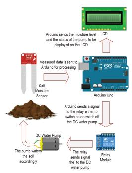
Fig. 2. The system architecture of the Automatic Irrigation System
