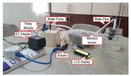
Fig. 5. Hardware implementation for the automatic irrigation system (Side view)
