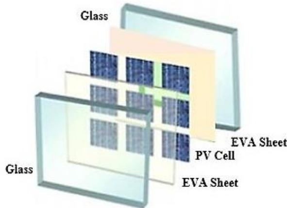
Fig. 9 – A simplified diagram of a of (STPV) structure
