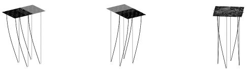
Mode 1 Mode 2 Mode 3 Figure 8.17: The first three mode shapes from the finite element model of the small platform
