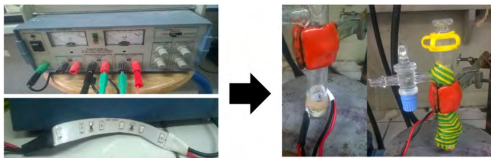
Figure 1.15 The set-up of thiol-ene reaction with the strip light, 5 UV light dots (365 nm).
