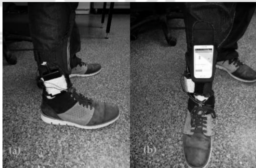
Figure 2: Positioning of the enactive insole on the foot: (a) signal amplifier is fixed on the ankle; (b) Enactive insole is wear into the shoe.
