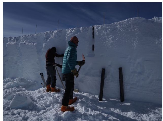
Figure 3. Sampling procedure in the OIR trench. The first carbon fiber tube (liner) is pushed into the snow after excavation of the trench. The positions were marked with a small bamboo pole. After retrieval of the first profile, the vertically consecutive second and third liners were taken. Two empty liners lean at the trench wall. The last liner had to be dug out partly as the trench was only 2 to 2.5 m deep.
