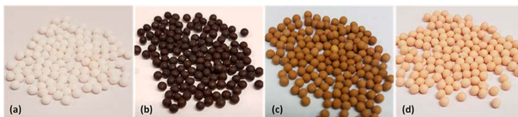
Figure 2. Pictures of (a) the native alumina particles and (b–d) the HQ-alumina composites obtained after drying, using an impregnation solution with (b) no additive, (c) \text{Na}_2\text{SO}_3 , and (d) \text{H}_2\text{SO}_4 .
