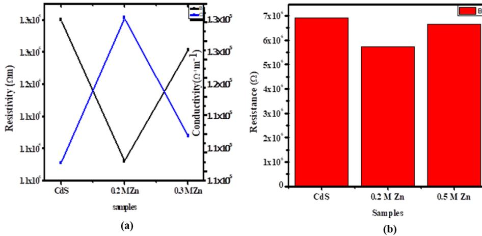
FIGURE 6. (a) Variation resistivity and conductivity of un-doped and metal-doped CdS nanoparticles and (b) Bar graph of resistance for un-doped and Zn-doped CdS nanocrystals
