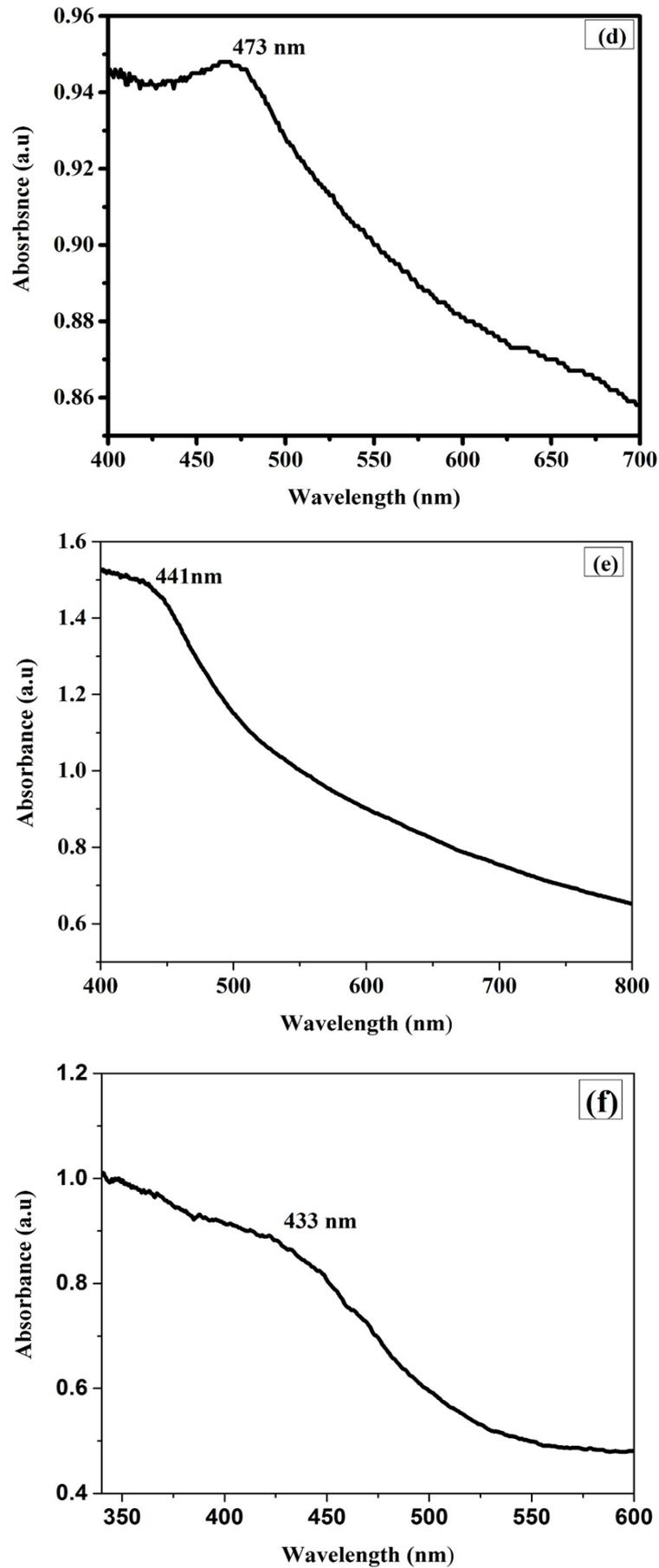
FIGURE 1. UV-visible spectra of (a) un-doped CdS, (b) 0.1 M Zn-doped CdS, (c) 0.2 M Zn-doped CdS, (d) 0.3 M Zn-doped CdS, (e) 0.4 M Zn-doped CdS, (f) 0.5 M Zn-doped CdS
