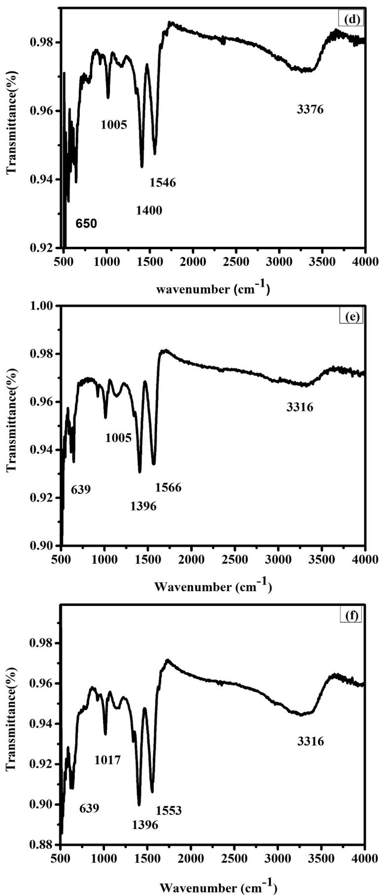
FIGURE 3. FTIR spectra of (a) un-doped CdS, (b) 0.1 M, Zn-doped CdS, (c) 0.2 M, Zn-doped CdS, (d) 0.3 M, Zn-doped CdS, (e) 0.4 M, Zn-doped CdS, (f) 0.5 M, Zn-doped CdS
