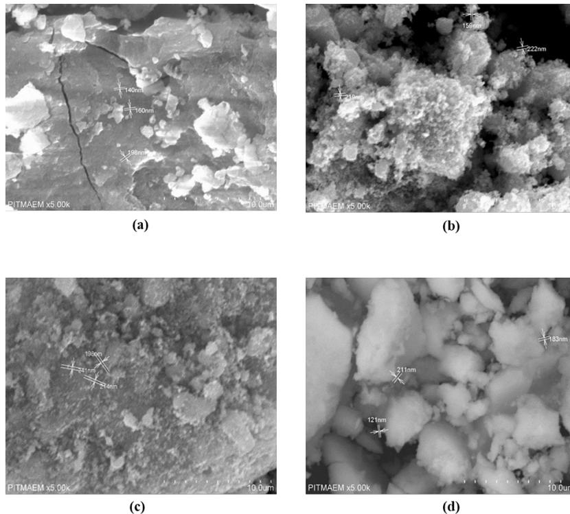
FIGURE 7. SEM images of (a) un-doped CdS, (b) 0.1 M, Zn-doped CdS, (c) 0.3 M, Zn-doped CdS, and (d) 0.5 M, Zn-doped CdS
