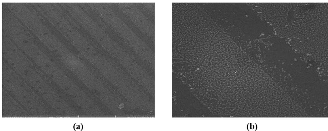
FIGURE 8. SEM images of (a) 0.5 M Zn-doped CdS pattern by  $\mu$ TM technique with low and (b) high resolution
