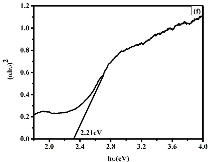
FIGURE 2. Tauc plot for (a) un-doped CdS, (b) 0.1 M Zn-doped CdS, (c) 0.2 M Zn-doped CdS, (d) 0.3 M Zn-doped CdS, (e) 0.4 M Zn-doped CdS, and (f) 0.5 M Zn-doped CdS
