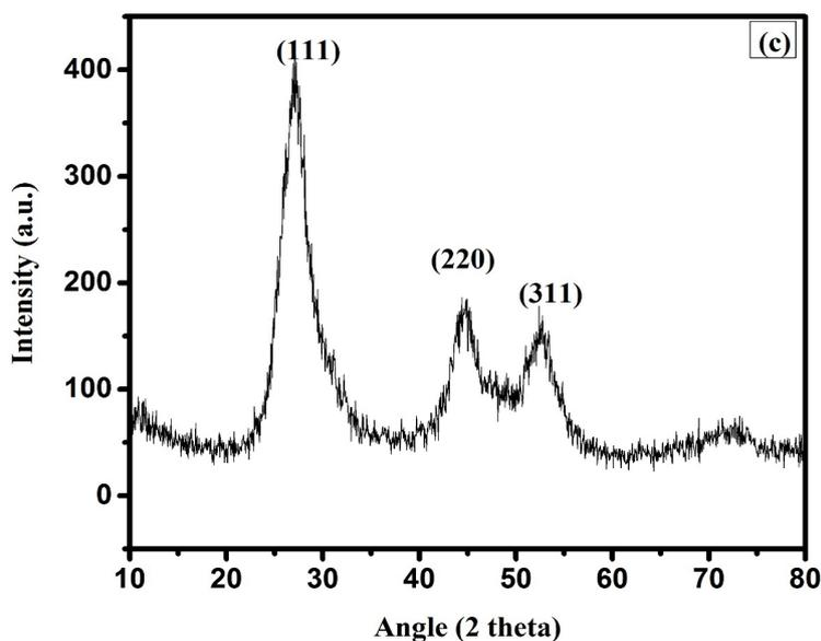
FIGURE 4. XRD pattern of (a) un-doped CdS, (b) Zn-doped CdS (0.2 M) and (c) Zn-doped CdS (0.4 M) nanocrystals
