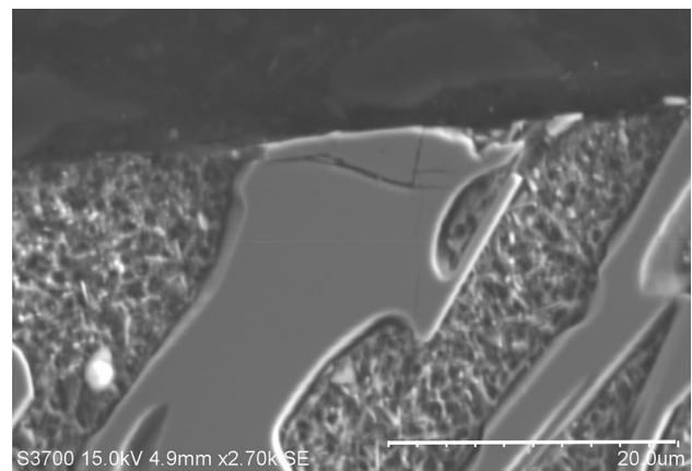
Fig. 20 Cracking in primary carbide in 27%Cr cast iron wear scar
