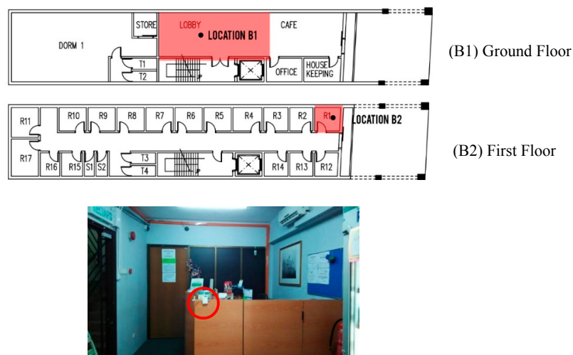
Figure 5. Location of data loggers in Building B.
