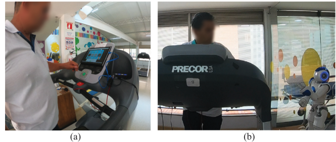
Fig. 1. Setup of the system for cardiac rehabilitation programme at Fundacin Cardioinfantil-Instituto de Cardiologia (Bogotá, Colombia): patient interacting with the (a) tablet interface, (b) personalised assistive robot.
