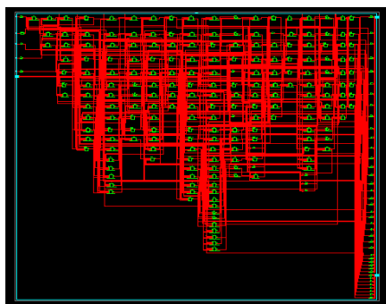
Fig 4: Simulation Technology schematic of crc Block replaced by XOR gate in ETI architecture
