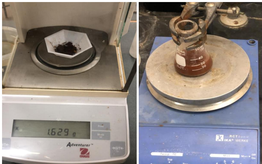
Figure 5-6: : Preparation of 0.5 M FeCl_3 in 0.1 M HCl.
