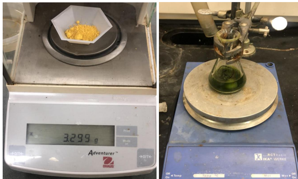
Figure 5-5: Preparation of 0.5 M K_3Fe(CN)_6 in 0.1 M HCl.
