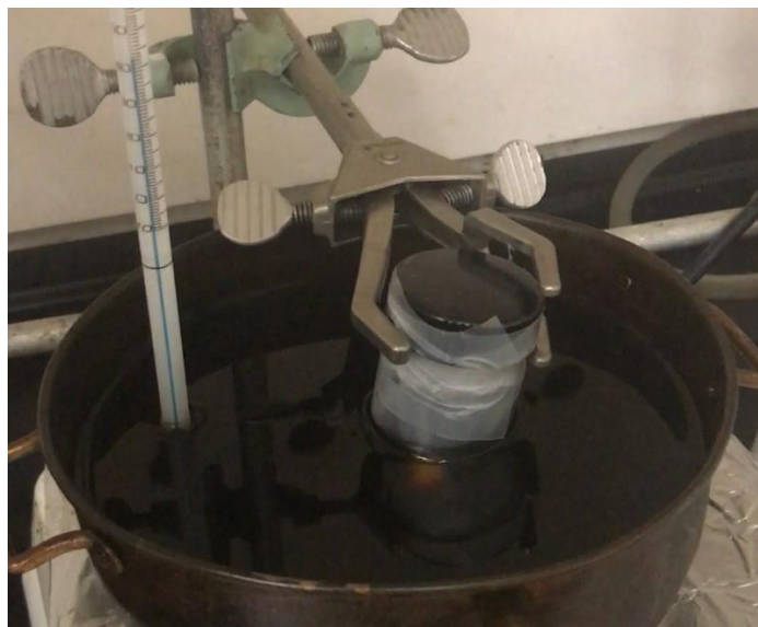
Figure 4-8: PVDF solution preparation.
