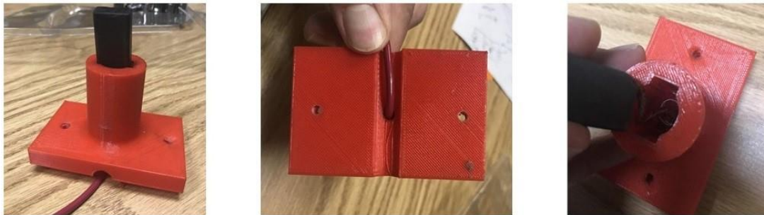
a) the position of carbon brush, spring and the accessibility of wire in 3D printed brush holder
