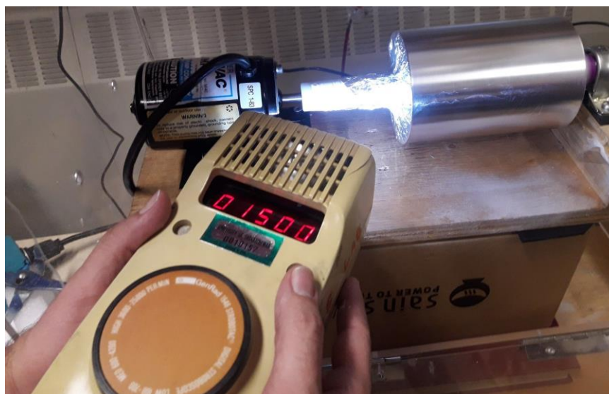
Figure 4-6: An illustration of drum speed control using the stroboscope technique.
