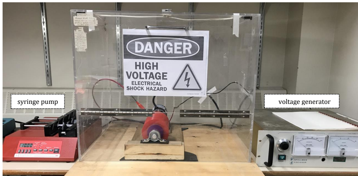
Figure 4-7: An illustration of assembled electrospinning machine.
