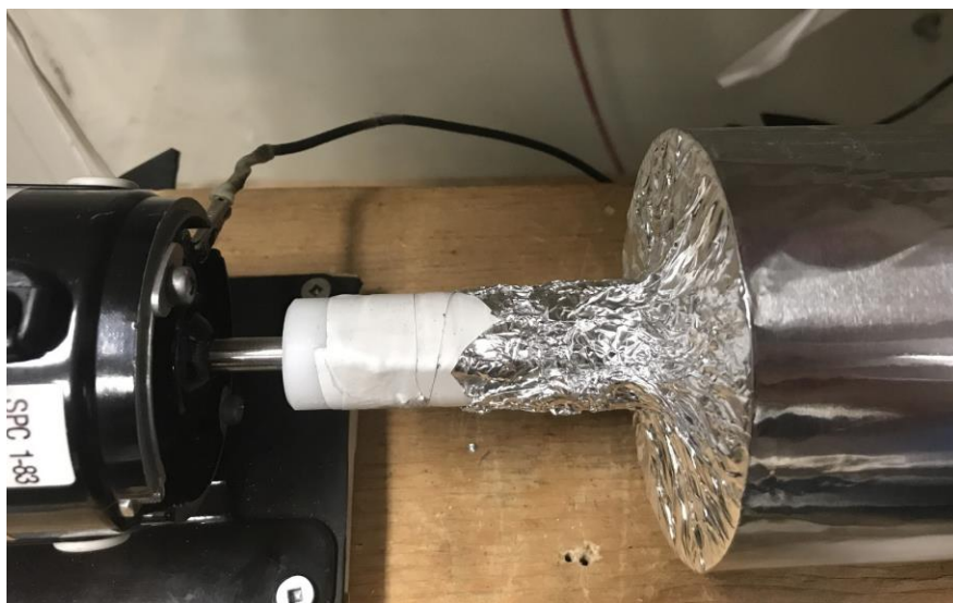
Figure 4-5: Connection and testing of drum conductivity through the motor shaft.
