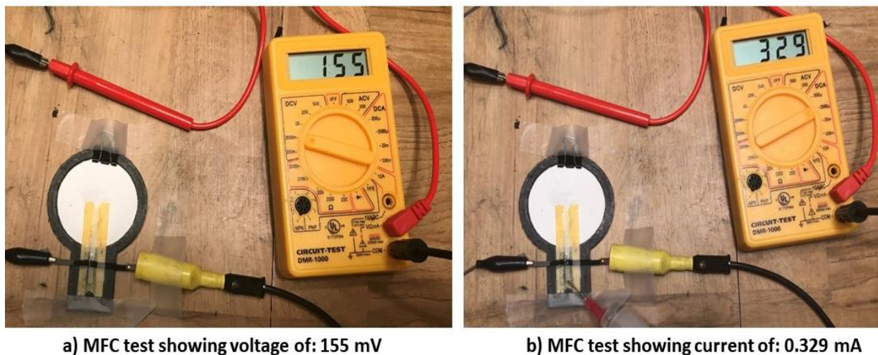
Figure 5-10: MFC electrochemical test results: a) showing voltage of 155 mV, and b) showing current of 0.329 mA.
