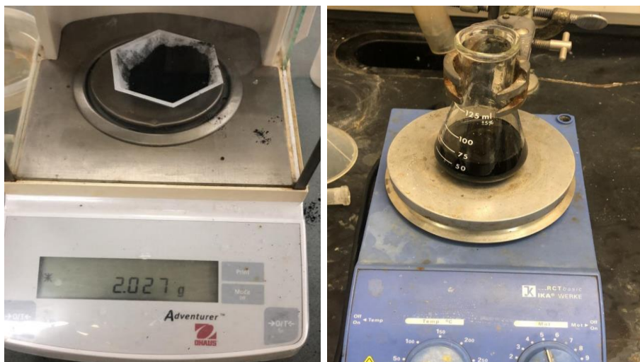
Figure 5-7: Suspension and agitation of carbon powder in 0.5 M K_3Fe(CN)_6 in 0.1 M HCl and 0.5 M FeCl_3 in 0.1 M HCl solutions.
