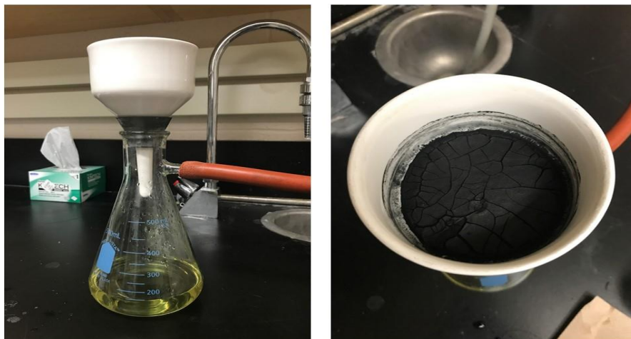
Figure 5-8: PB supported by carbon powder filtration process.
