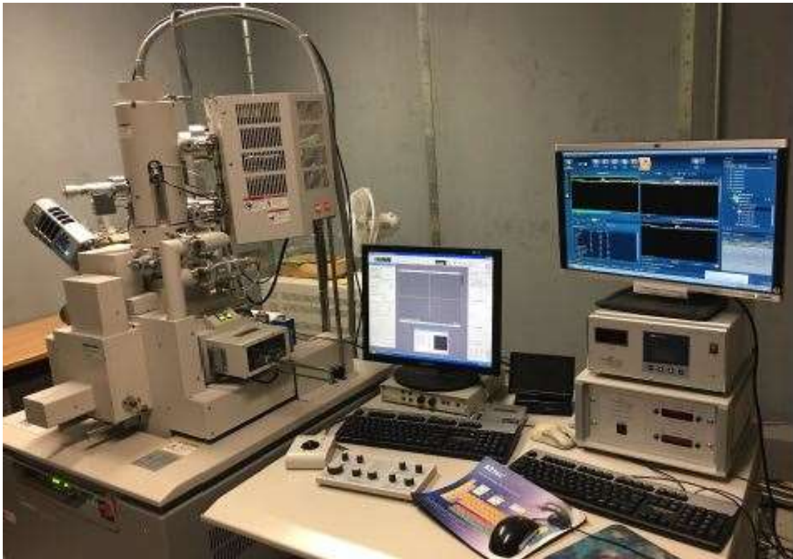
Figure 3.5: Hitachi Field Emission (SU 6600) SEM equipped with an Oxford Instruments NordlysNano EBSD and EDS at the material science laboratory, University of Saskatchewan.
