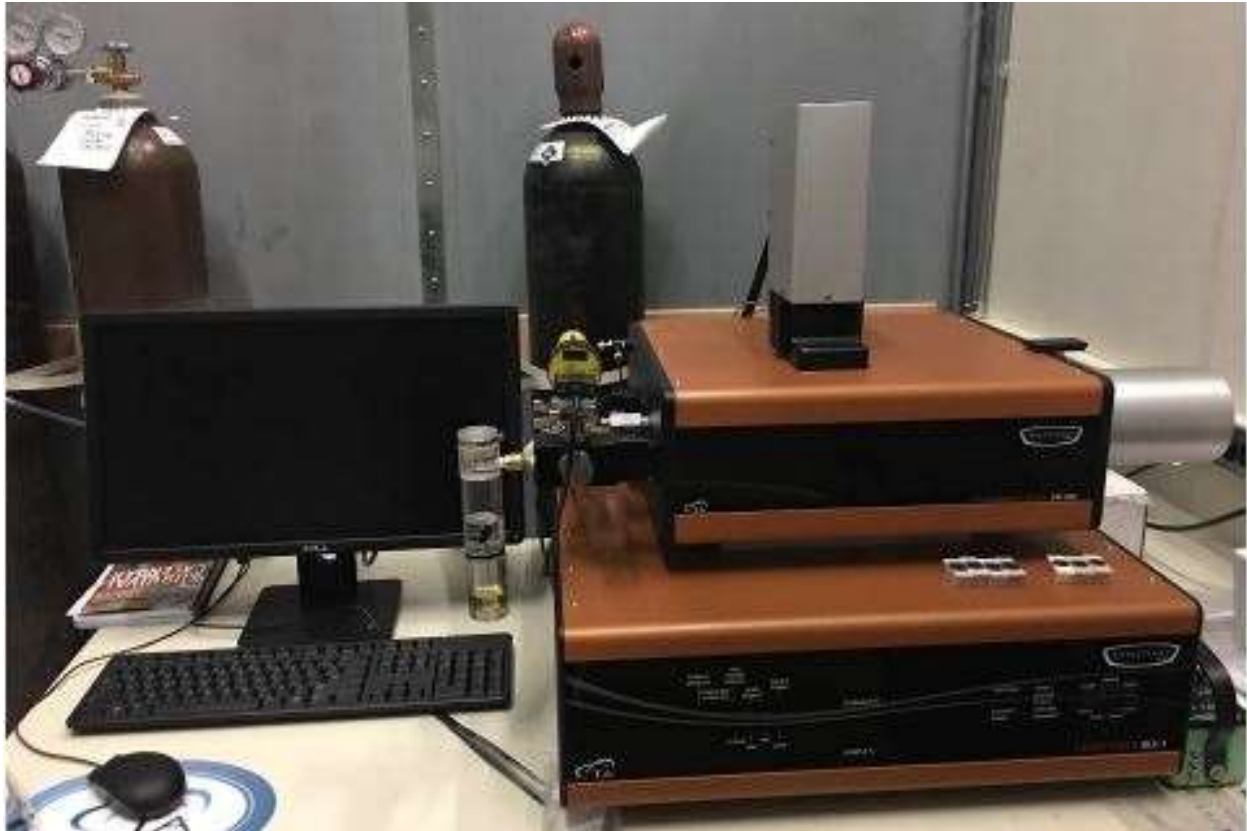
Figure 3.7: Laser flash equipment (DLF-1/EM-1300) from TA Instruments at the material science laboratory, University of Saskatchewan.
