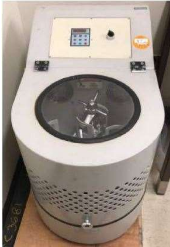
Figure 3.1: Planetary ball mill (Torrey Hills-ND2L) at the material science laboratory, University of Saskatchewan.
