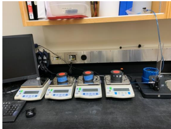
Figure 3-2: Laboratory set-up for measuring the SMC of the silica sand using the HYPROP equipment
