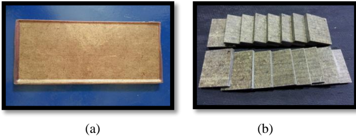
Figure 2: (a) Kenaf fiber reinforced plastic board, (b) sample for experiment
