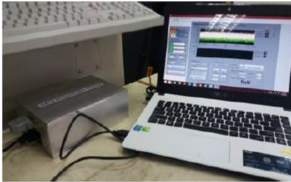
Figure 2: Neo MoMac cutting force measuring system
