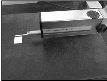
Figure 3: Surface analyzer for measuring surface roughness (Perthometer S2 PGK)
