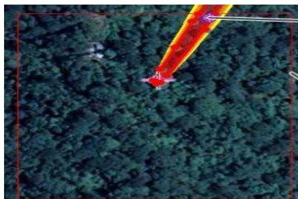
Fig. 10: Footprint of toxicity of MeOH, Plant 2– night, 25 mm leakage, 2% fatality (from SSW wind direction).
