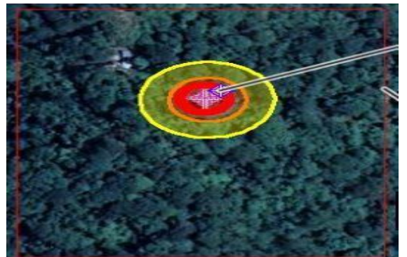
Fig. 7: Footprint of jet fire from MeOH, Plant 1–day, 160 mm leakage, 1% fatality
