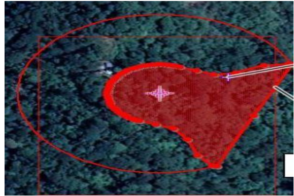
Fig. 4: Puff dispersion at Plant 1–release of CO 2 at night, 160 mm leakage, 27% fatalities (from WNW wind direction).
