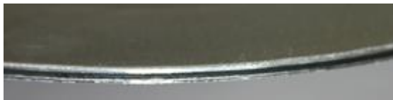
Figure 2: Pre-consolidated FML specimen
