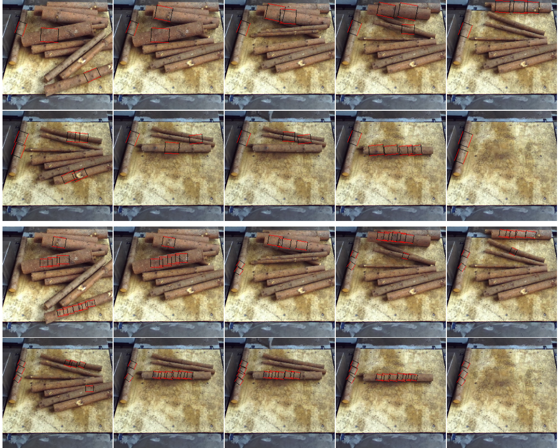
Figure 7. Comparison of predicted grasping candidates for both networks trained on automatically labeled data ( top two rows ) and manually labeled data ( bottom two rows ). We apply non-maximum suppression to reduce the number of visualized boxes and to ensure the clarity of the visualization.
