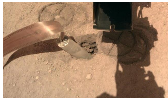
Figure 2: Arm camera image of the hole excavated by the HP 3 mole. The mole end is ~5 cm above the surface.
