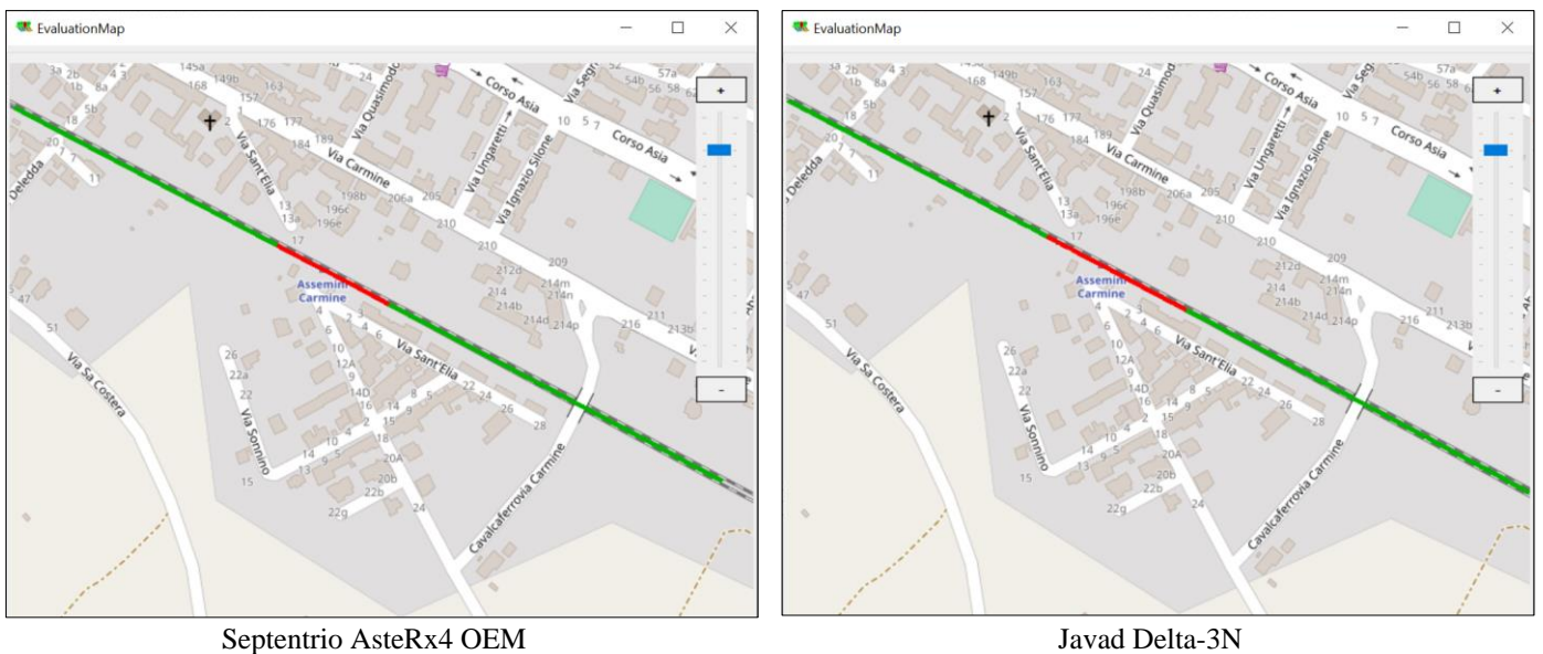
Figure 12: Comparison of the interference detection results at Assemini station
