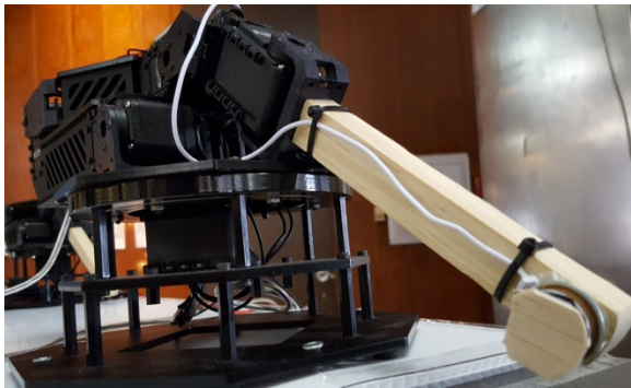
Figure 17: Touchbot #2 : User's controller #2 with vibration speaker and wood chip pad on end.
