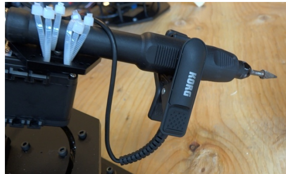
Figure 18: Touchbot #2 : Korg high fidelity contact microphone on Dremel tool (© Morgan Rauscher).
