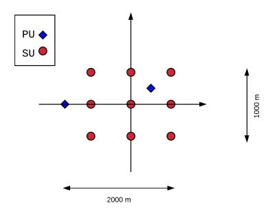
Figure 4.6: The network deployment for the n=9 cooperation size and m=2 PUs.
