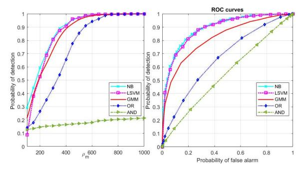
Figure 3.8: The probability of detection for different values of  $\rho_m$  at a probability of false alarm of 0.1 and the corresponding ROC curves.
