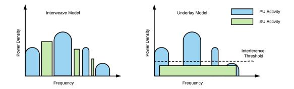
Figure 2.3: Dynamic spectrum access for the interweave and underlay CR access models.
