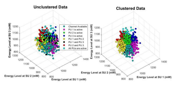
Figure 3.5: Multi-class SVM before and after training for scenario-II for a PU transmit power  $\rho_m = 80$  mW.
