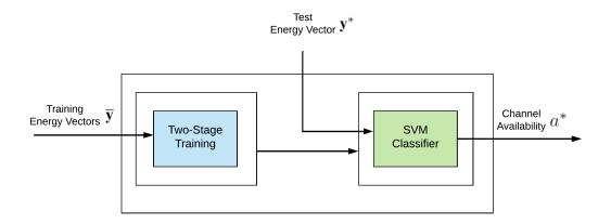
Figure 4.5: Two-Stage learning-based spectrum sensing block diagram.
