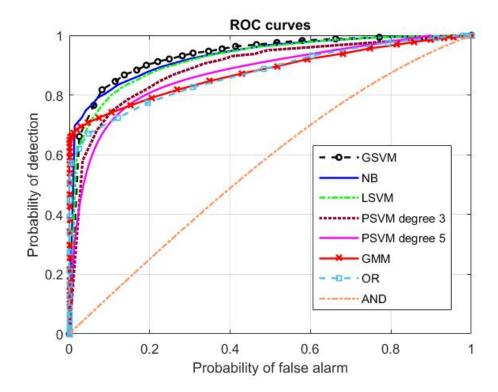
Figure 3.7: The ROC curves at  $\rho_m = 200$  mW.
