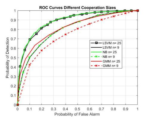
Figure 3.10: Examining the effect of increasing the cooperation size n while sensing a single PU with  $\rho_m = 200$  mW.
