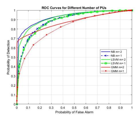
Figure 3.9: Examining the effect of increasing the number of PUs m, each transmitting with  $\rho_m = 200 \text{ mW}$ .
