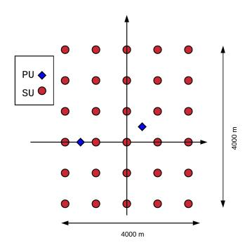
Figure 3.6: The node deployment in the proposed CR network in scenario-I.
