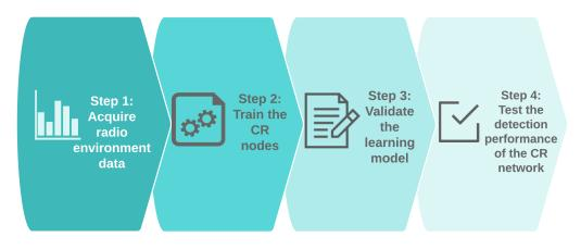
Figure 3.1: Stages of establishing a machine learning model for cooperative CR networks.
