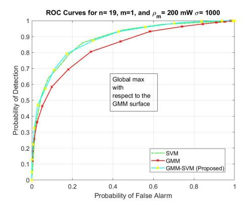
Figure 4.9: Performance analysis in the case where the GMM surface achieves a global maxima.
