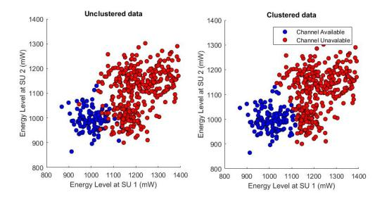
Figure 3.2: Classification using the GMM algorithm for scenario-*I*.
