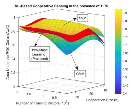
Figure 4.7: The joint effect of the number of training vectors and the size of the secondary network when m = 1.
