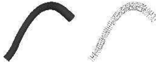
Fig. 3: Example of a RGC-sm. Left: Surface representation. Right: Stack of contours. Note the presence of the generating axis.
