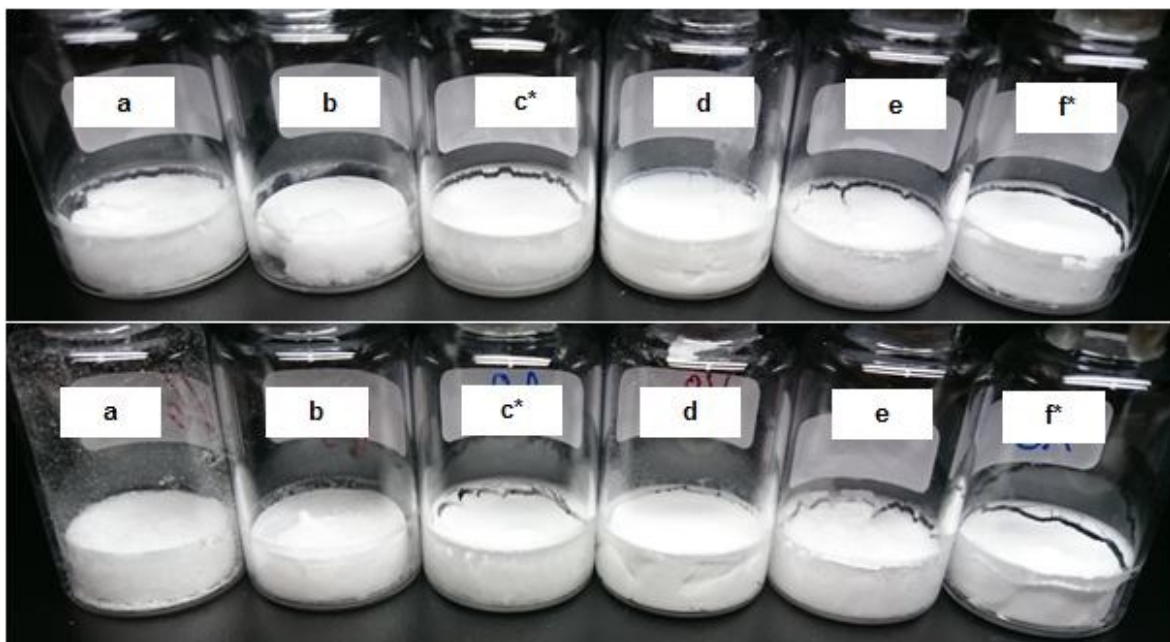
Figure II-1 Representative photographs of differently dried formulations. Small letters represent the excipient used: a 10% sucrose, b 1% sucrose, c 10% trehalose, d 10% mannitol:sucrose 4:1, e 10% HP- \beta -CD:sucrose 1:1, f arginine phosphate. Top picture : CFD-products; Bottom picture : MFD-samples. The asterisk indicates that these formulations contained 5 g/L mAb and were dried in a separate but similar run to the one shown in Figure II-2.
