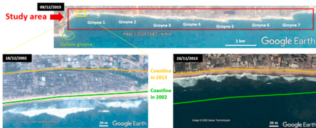
Fig. 2. Evolution of the coastline in the Western part of the study area between 2002 and 2013.
