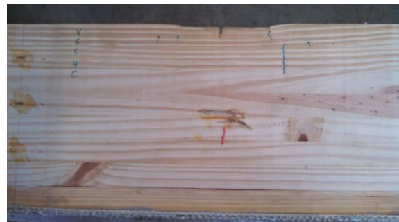
Figure 17. Compressive region of the beam and the failure of the upper lamellas in bending test.
