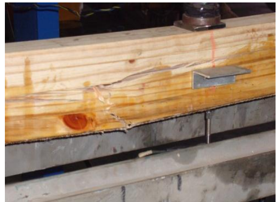
Figure 16. Region of the mid-span of the beam and the failures of the lamellas and Sisal fibres in bending test.
