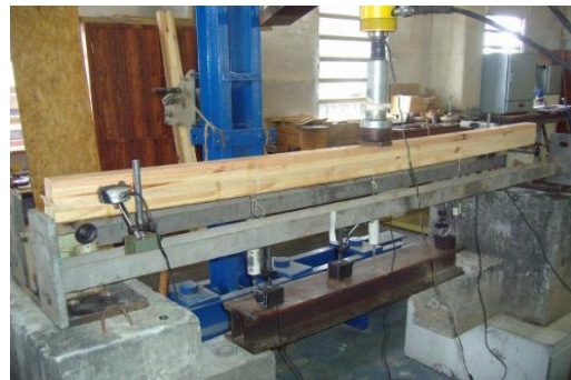
Figure 10. Glued laminated timber beam for bending test.
