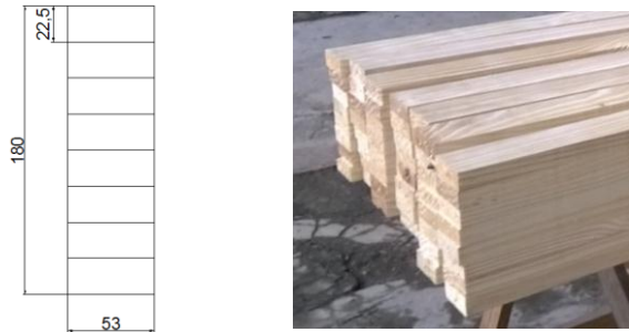
Figure 8. Scheme of the cross section (dimension in mm) and the layers to manufacture the beams.
