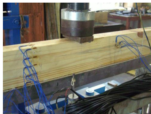
Figure 11. Central region of the beam positioned for testing with strain gauges positioned in its section.
