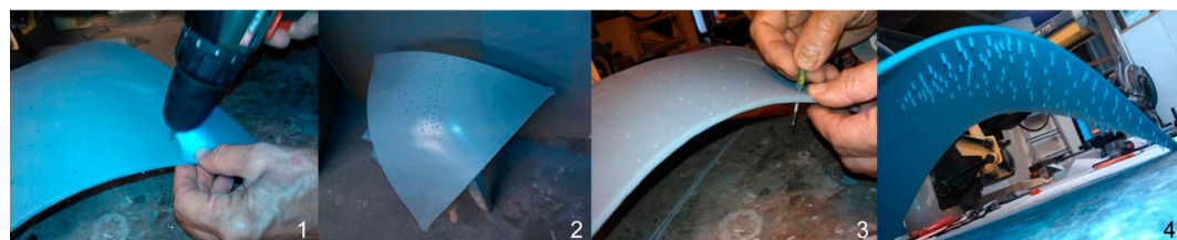
Figure 11. Installation of pressure sensors: (1) drilling; (2) painting with coating; (3) installation of pressure sensors; and (4) final instrumented model.
