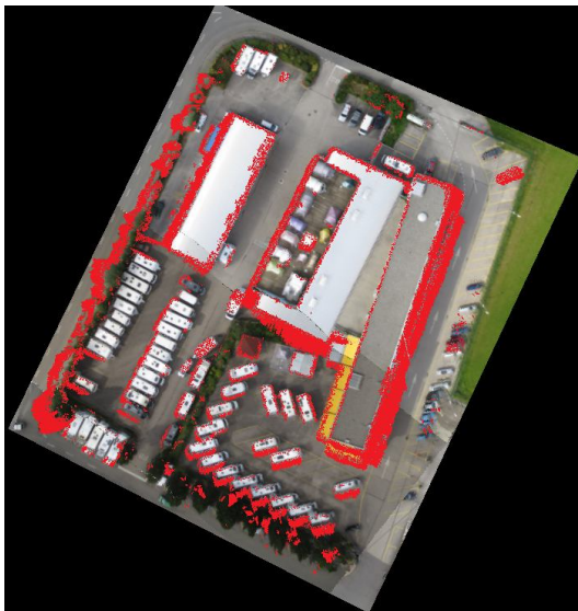
Figure 8. Occlusion detection for the area of interest based on the proposed approach - HGM.
