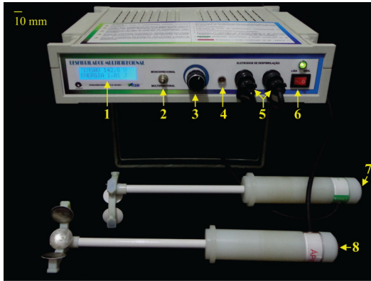
Figure 3. The multidirectional defibrillator and the paddles. From the left to the right in the instrument’s control panel: (1) display that shows the charged voltage and energy level; (2) switch for selection of shock delivery modality; (3) rotary potentiometer for adjusting shock energy; (4) LED that indicates stimulus delivery; (5) outputs for connection to the electrode cables; and (6) on/off switch. Each paddle bears 3 electrodes, which allow shock delivery in 3 directions spaced by 60° (see text for details). Labeled pushbuttons on the top of each handle enable capacitor charging (7) or discharge triggering (8).
