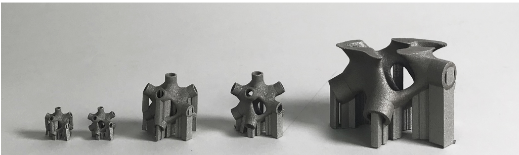
Figure 2.13: Physical experiments of 3D printed nodal connection in steel created with powder bed laser fusion printing. The shape of the node is found through a topology optimisation process as described in [4]. Photo taken by the author.
