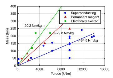
Fig. 1.17: Mass of different large direct-drive generators as a function of the torque from Table 1.7.
