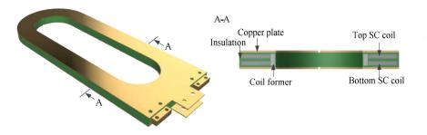
Fig. 6.18: Structure of the superconducting double pancake coil.
