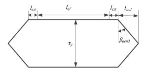
Fig. 2.3: Sketch and main dimensions of an armature coil.
