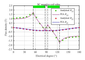
Fig. 3.14: Comparison of FEA and analytical results of the magnetic flux density under rated load in the superconducting coils.
