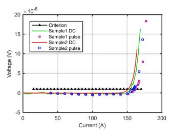
Fig. 6.6: Comparison of critical current in liquid nitrogen with DC current supply and pulse current supply.
