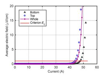
Fig. 6.21: Simulated average electric field as a function of the supply current.
