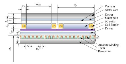
Fig. 2.1: Dimension parameters in a superconducting DC generator.
