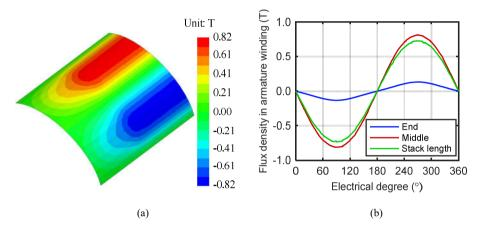
Fig. 5.6: Radial component of flux density in the armature winding: (a) flux density distribution in the middle radial position, (b) flux density at different axial positions.
