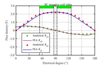
Fig. 3.10: Comparison of FEA and analytical results of flux density in stator iron yoke under no load.
