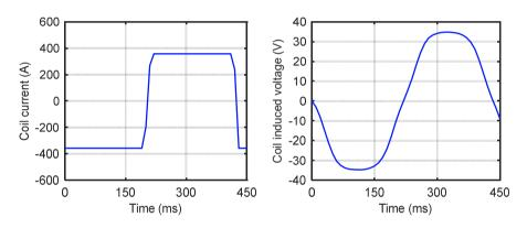
Fig. 7.5: Current and induced voltage of one coil of the superconducting DC generator.
