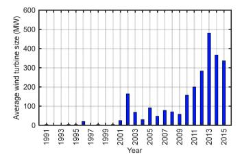
Fig. 1.5: Average offshore wind turbine size installed from the year 1991-2015 [15].
