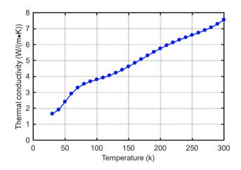
Fig. 5.16: Calculated thermal conductivity of the titanium alloy Ti6Al4V.
