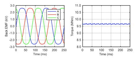
Fig. 7.13: Induced voltage at no load and torque at rated load of the copper coil excited generator.
