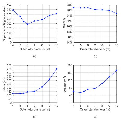
Fig. 7.16: Superconducting tape length, efficiency, mass and volume as a function of outer rotor diameter.
