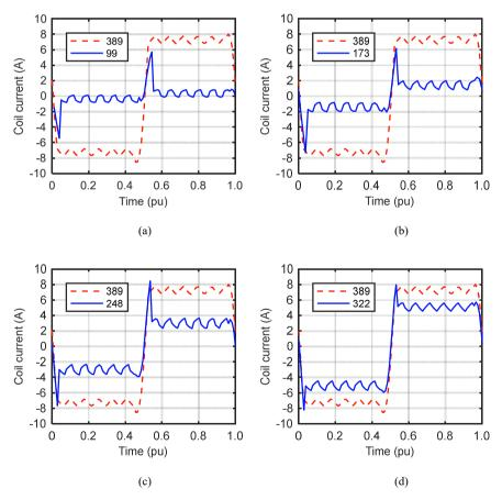
Fig. 5.22: Current per coil at different rotational speeds with brush shift 3.2°, (a) 99 (1/min), (b) 173 (1/min), (c) 248 (1/min), and (d) 322 (1/min).
