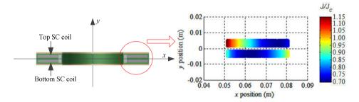
Fig. 6.22: Current density distribution of one superconducting coil side under critical current of 45.9 A.
