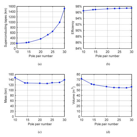
Fig. 7.17: Superconducting tape length, efficiency, mass and volume as a function of pole pair number.
