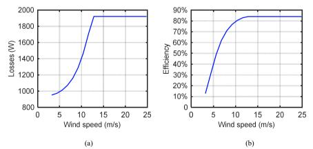
Fig. 5.26: Illustration of losses and efficiency of the generator with wind speeds, (a) losses, and (b) efficiency.
