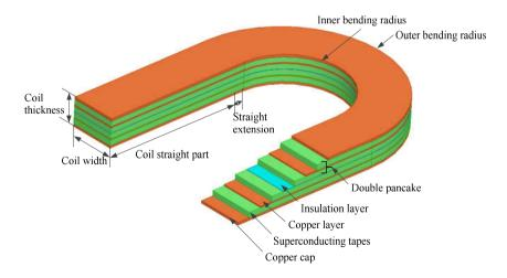
Fig. 5.9: Structure of the superconducting coil.
