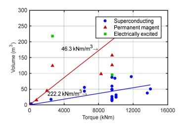
Fig. 1.18: Volume of different large direct-drive generators as a function of the torque from Table 1.7.
