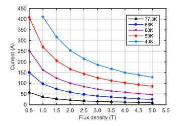
Fig. 6.9: Magnetic field dependence of the tape @ Superpower with the angle of 45°.
