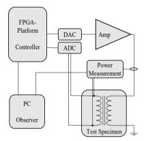
Fig. 6.12: Sketch of measurement system.
