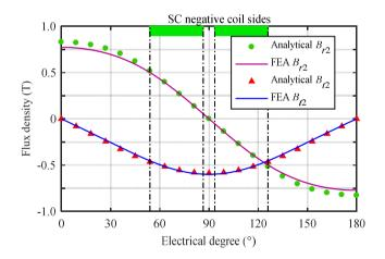
Fig. 3.8: Comparison of FEA and analytical results of flux density in physical air gap under no load.
