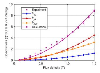
Fig. 6.16: Iron loss model of M235-35A at 100 Hz and 77 K ( $h_{ec}$  is the eddy current loss,  $h_{ys}$  is the hysteresis loss, and  $h_{exc}$  is the excess loss ).
