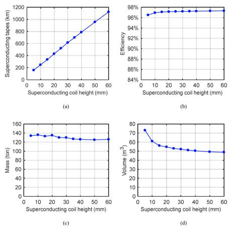
Fig. 7.18: Superconducting tape length, efficiency, mass and volume as a function of superconducting height.
