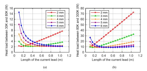
Fig. 5.19: Heat loss of one current lead with different lengths and diameters,(a) Heat load between 30 K and 80 K, and (b) heat load between 80 K and 300 K.
