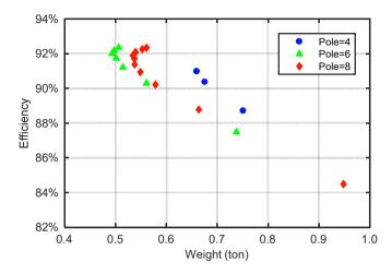
Fig. 5.4: Influence of the pole pair number on the major design parameters of the generator.
