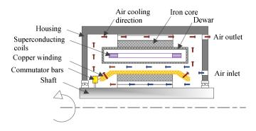
Fig. 5.12: Sketch of axial forced air cooling.
