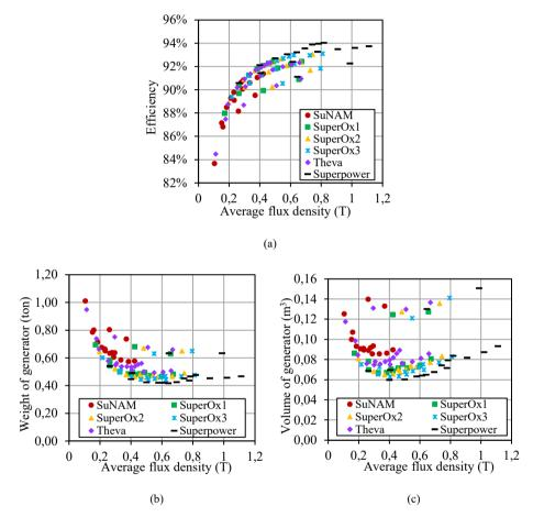
Fig. 5.3: Major design parameters as a function of the average air gap flux density of the 10 kW generator with different tapes, (a) efficiency of the generator (refrigeration losses is not included), (b) weight of the generator, and (c)overall volume of the generator.
