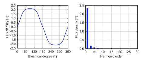
Fig. 7.3: Flux density distribution of the armature winding (in the middle position in radial direction) and its harmonic spectrum of the superconducting DC generator.
