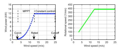
Fig. 5.20: Sketch of wind power and rotor speed with wind velocities.
