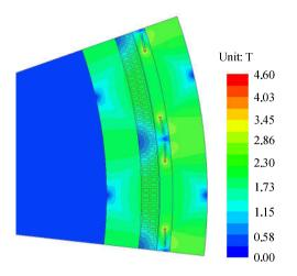
Fig. 7.2: Flux density distribution of the one pole pair model of the superconducting DC generator.
