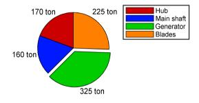
Fig. 1.16: Distribution of the tower head mass for a 10 MW permanent magnet wind turbine generator[80].
