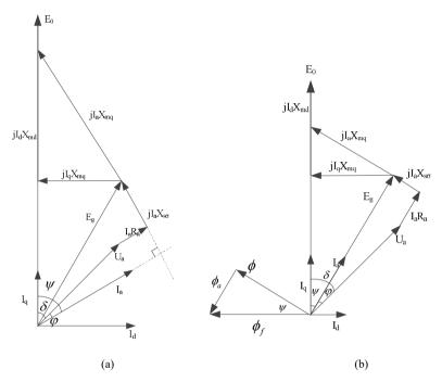
Fig. A.4.2: Phasor diagram, (a) general phasor diagram, and (b) phasor diagram with  $I_a$  and  $E_g$  in-phase.
