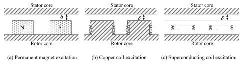
Fig. 1.6: Different pole excitation methods.
