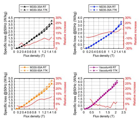
Fig. 6.14: Iron loss of the four different samples at 50 Hz.
