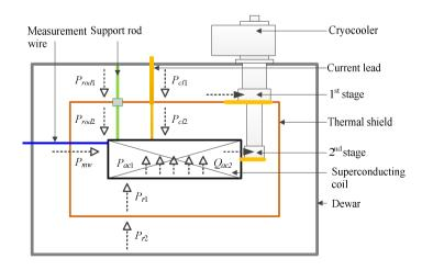
Fig. 5.13: Heat loads at cold temperature.
