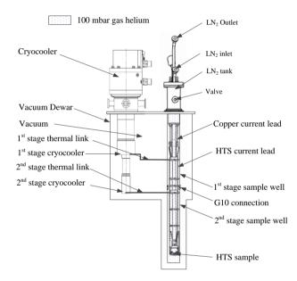
Fig. 6.2: Cryostat of the sample holder.
