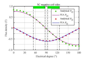
Fig. 3.13: Comparison of FEA and analytical results of the flux density under rated load in the air gap.
