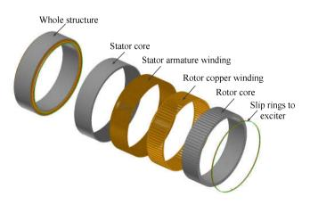
Fig. 7.14: Three-dimensional view of the copper coil excited generator.
