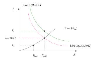
Fig. 2.9: Operating current of a superconducting coil @ H//c.
