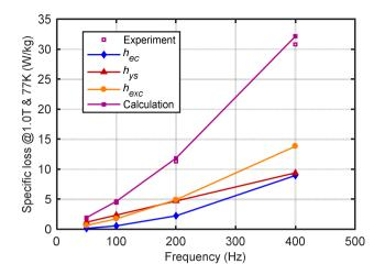
Fig. 6.17: Iron loss model compared with experiment data of M235-35A at 1.0 T and at liquid nitrogen temperature ( $h_{ee}$  is the eddy current loss,  $h_{ys}$  is the hysteresis loss, and  $h_{eve}$  is the excess loss).
