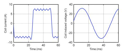
Fig. 5.8: Coil current and voltage of the generator.
