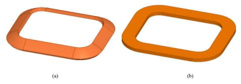
Fig. 3.15: 3D superconducting coil in the analytical model and in practice, (a) analytical model, (b) in practice.
