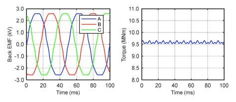
Fig. 7.9: No-load induced voltage and rated torque of the PM generator.
