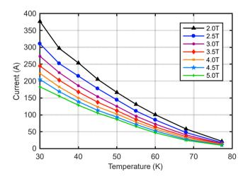
Fig. 6.8: Temperature dependence of the tape @ Superpower with the angle of 45°.
