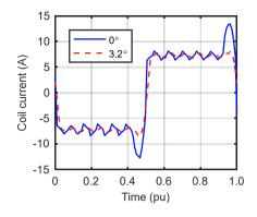
Fig. 5.21: Current per coil with/without brush shift at rated rotational speed.
