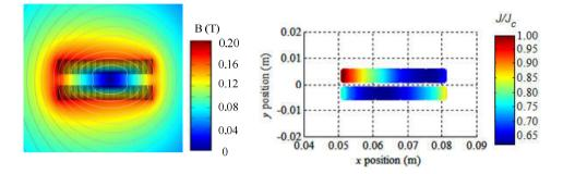
Fig. 6.23: Flux and current density distribution of one superconducting coil side under critical current of 42.3 A.
