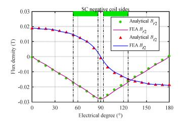
Fig. 3.11: Comparison of FEA and analytical results of the magnetic flux density generated by armature winding in the air gap.
