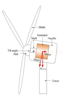
Fig. 4.3: Sketch of the tilt angle and gravity components of the superconducting generator.
