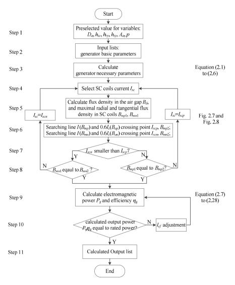
Fig. 2.5: Flowchart of design process.
