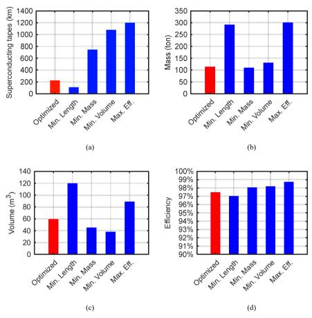
Fig. 7.1 Optimization results based on different objectives, (a) minimal superconducting wire length, (b) minimal mass, (c) minimal volume, and (d) maximum efficiency.
