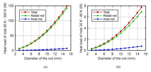
Fig. 5.17: Heat load of the tie rods when the diameter of the rods is varied,(a) temperature between 80 K and 300 K, and (b) temperature between 30 K and 80 K.
