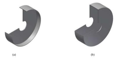
Fig. 4.4: Support structure of the generator, (a) rotor support, and (b) stator support.
