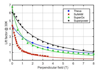
Fig. 5.2: Simulation of lift factor at 30 K for different tapes.
