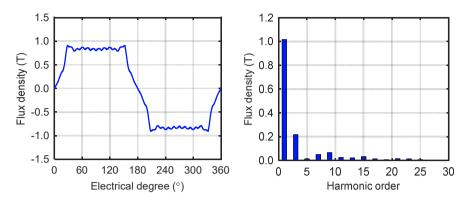
Fig. 7.12: Flux density distribution of the air gap and its harmonic spectrum of the copper coil excited generator.
