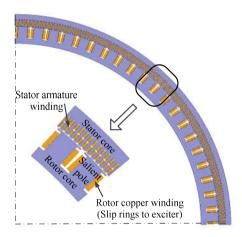
Fig. 1.8: Sketch of an electrically excited direct drive synchronous generator.
