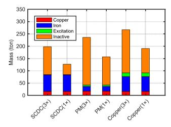
Fig. 7.15: Component masses of the three generators when the inactive materials of the generators are calculated based on rated torque and 3 times rated torque, respectively.
