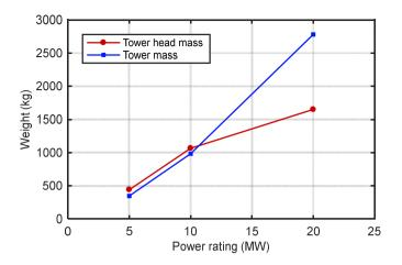
Fig. 1.15: Mass estimation for 5, 10 and 20 MW wind turbines of permanent magnet generators [59].
