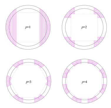
Fig. 3.17: Cross section of the superconducting coils with different coil layers and pole pairs.
