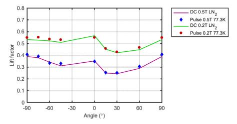
Fig. 6.7: Comparison of lift factor between pulse and DC current supply at 0.2 T and 0.5 T, respectively.
