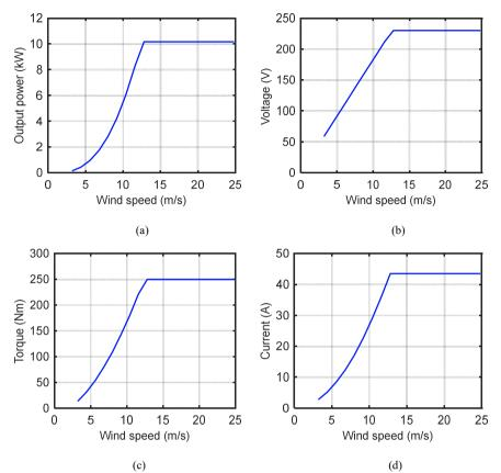
Fig. 5.25: Illustration of the power, voltage, current, and torque of the generator with different wind speeds, (a) Output power, (b) Voltage (c) Torque, and (d) Current.
