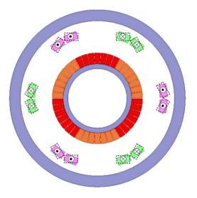
Fig. 3.16: Difference of the cross section in the analytical model and in practice, the dashed line is the cross section in practice.
