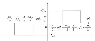
Fig. 3.5: Armature winding turns density of slot pair *j/j* ' per pole pair.
