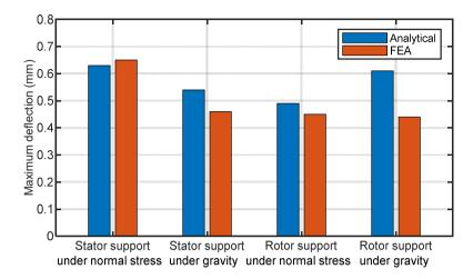
Fig. 4.5: The maximum deflection calculated by FEA and analytical model for stator and rotor support.
