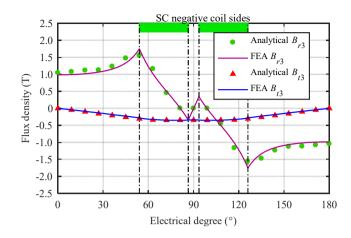
Fig. 3.9: Comparison of FEA and analytical results of flux density in superconducting coils under no load.
