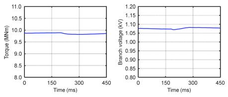
Fig. 7.4: Torque and branch voltage at rated load of the superconducting DC generator.
