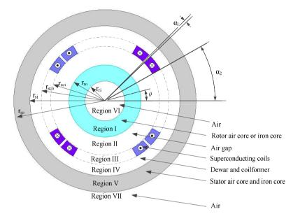
Fig. 3.1: General superconducting DC generator model.
