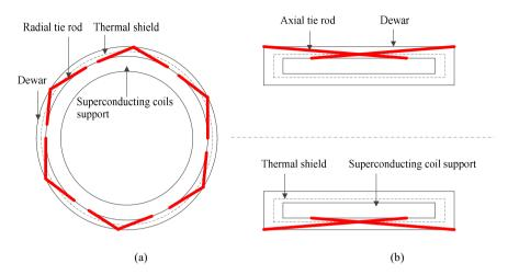
Fig. 5.15: Illustration of superconducting coil support, (a) radial rods, (b) axial rods.
