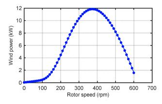
Fig. 5.1: Mechanical power cure with rotational speed.
