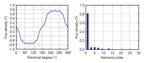
Fig. 7.8: Flux density distribution of the air gap and its harmonic spectrum of the PM generator.
