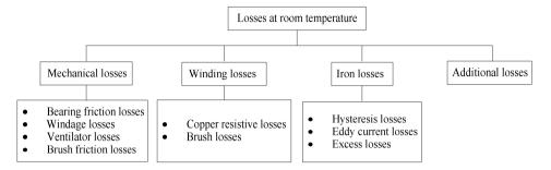
Fig. 5.11: General losses at room temperature of a superconducting generator.
