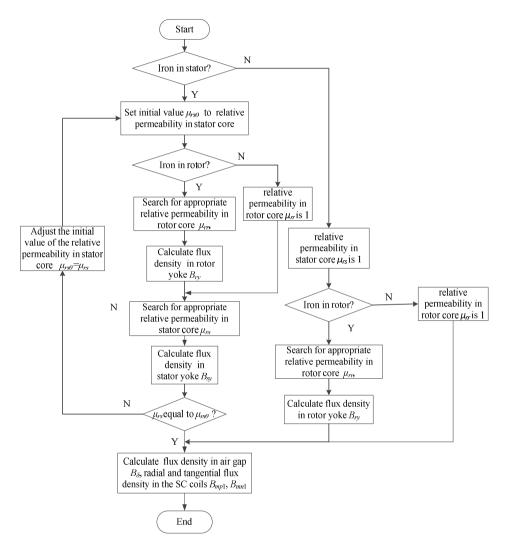
Fig. 2.6: Flowchart to calculate flux density in the generator.
