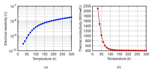
Fig. 5.18: The electrical resistivity and thermal conductivity of copper with RRR=100,(a) electrical resistivity, and (b) thermal conductivity.
