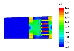
Fig. 7.7: Flux density distribution of the one pole model of the PM generator.
