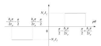
Fig. A.4.1 Magnetomotive force of one pole pair in the air gap.
