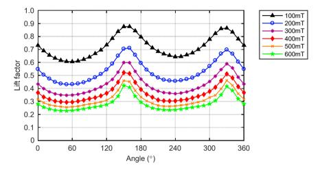
Fig. 6.20: Measured lift factor of the superconducting tape used in the coil in liquid nitrogen.
