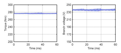
Fig. 5.7: Torque and branch voltage of the generator.
