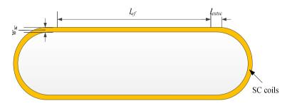
Fig. 2.4: Sketch and main dimensions of a superconducting coil.
