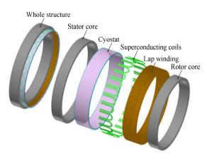
Fig. 7.6: 3D view of the superconducting DC generator (excluding commutator bars and brushes).
