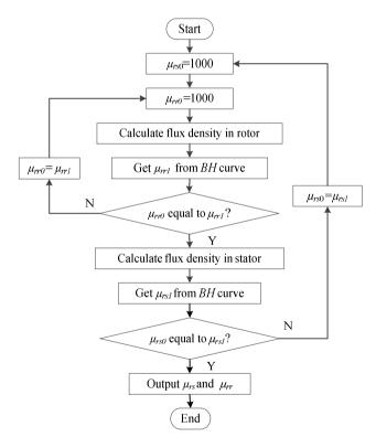
Fig. 3.3: Iterative algorithm to determine relative permeability.
