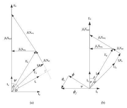
Fig. A.3.1: Phasor diagram, (a) general phasor diagram, and (b) phasor diagram with  $I_a$  and  $E_g$  in-phase.
