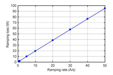
Fig. 5.14: Ramping loss with different ramp rates.
