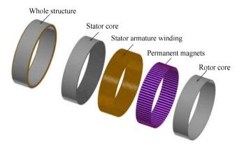
Fig. 7.10: Three-dimensional view of the PM generator.
