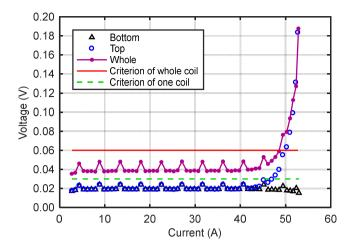
Fig. 6.19: Tested V-I curve of the superconducting double pancake coil in liquid nitrogen.
