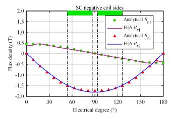
Fig. 3.7: Comparison of FEA and analytical results of flux density in rotor iron yoke under no load.
