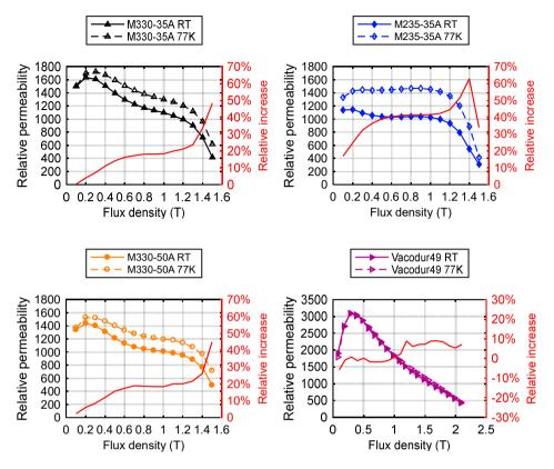
Fig. 6.13: Relative permeability of the four different samples at 50 Hz.
