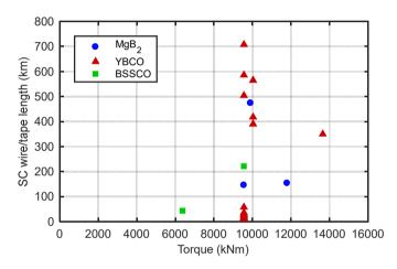
Fig. 1.20: Superconductor consumption as a function of torque from Table 1.7.
