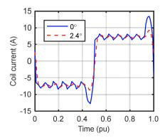
Fig. 5.23: Current per coil with brush shift 2.4° and without brush shift at rated rotational speed.
