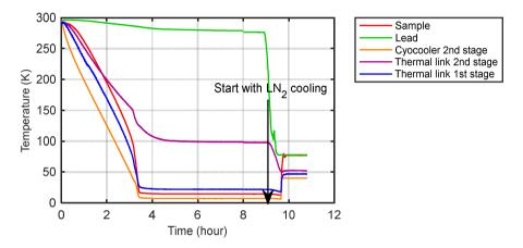
Fig. 6.4: Cooling down of the sample holder.
