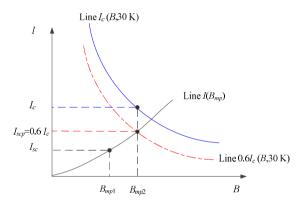
Fig. 2.8: Operating current of a superconducting coil @ H//ab.
