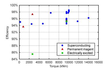
Fig. 1.19: Efficiency of different large direct-drive generators as a function of the torque from Table 1.7.
