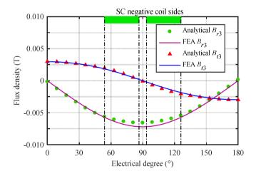
Fig. 3.12: Comparison of FEA and analytical results of the magnetic flux density generated by armature winding in the superconducting coils.
