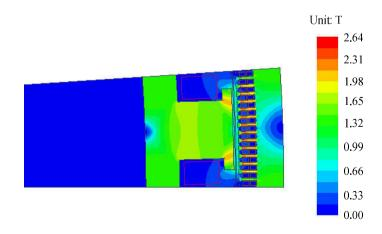
Fig. 7.11: Flux density distribution of the one pole model of the copper coil excited synchronous generator.
