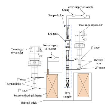
Fig. 6.1: Schematic overview of the system.
