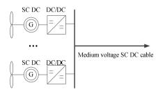
Fig. 1.1: Brief sketch of a superconducting DC generation and transmission scheme.
