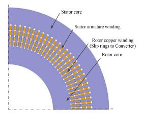
Fig. 1.7: Sketch of a doubly fed induction generator.
