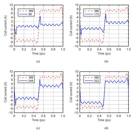
Fig. 5.24: Current per coil at different rotational speeds with brush shift 2.4°, (a) 99 (1/min), (b) 173 (1/min), (c) 248 (1/min), and (d) 322 (1/min).
