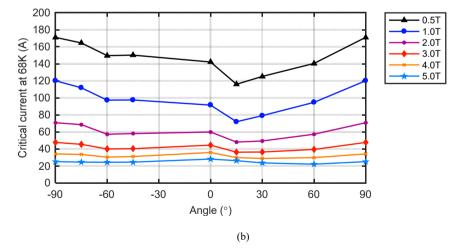
Fig. 6.10: Angular dependence of the tape from Superpower at 77.3K and 68K, respectively.
