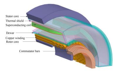
Fig. 5.5: A three-dimensional view of the generator (one pole pair model, excludes brushes).
