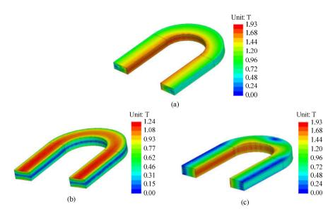
Fig. 5.10: Distribution of the magnetic field,(a) magnitude of the flux density,(b) magnitude of perpendicular component, and (c) magnitude of parallel component.
