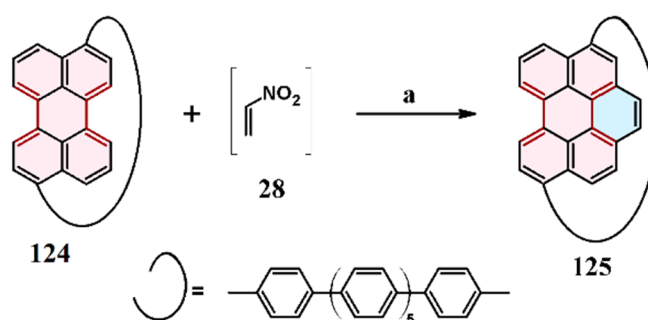
Scheme 29. Cycloaddition of acetylene generated in situ from nitroethanol to a cycloparaphenylene containing a perylene motif [148]. Reagents and conditions: (a) 2-nitroethanol (acetylene source), phthalic anhydride, 200 °C, MW, o -Cl 2 C 6 H 4 , 20 h.
