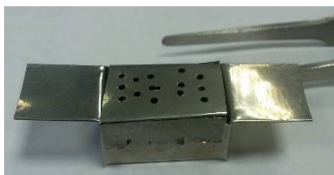
Fig. 2. Crucible with perforated cover used for calcium carbonate conversion in vacuum by resistant heating.
