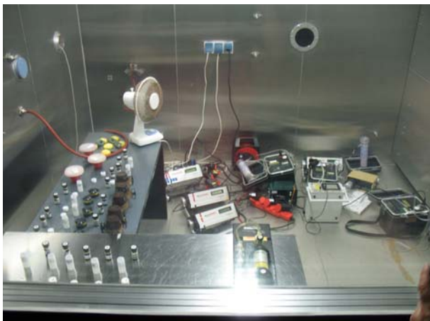
Fig. 2. The view of the interior of the radon chamber during the PTs.
